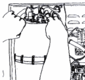
Place cylinder vertically into cylinder base
