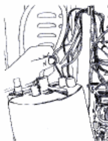
Connect plug to level sensor / electrodes
